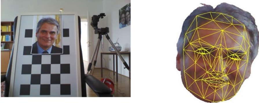
Figure 1: Face tracking from Kinect V1 image sample. Original image (left), Face texture w/ mesh (right, white=transparent)
