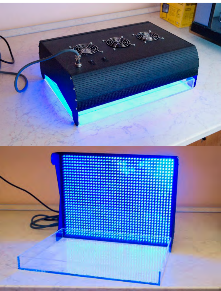
Fig. 2: Installation for light bleaching of paper with 1200 blue LEDs
