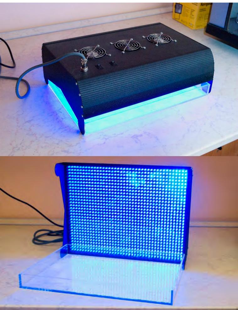
**Fig. 2:** Installation for light bleaching of paper with 1200 blue LEDs
