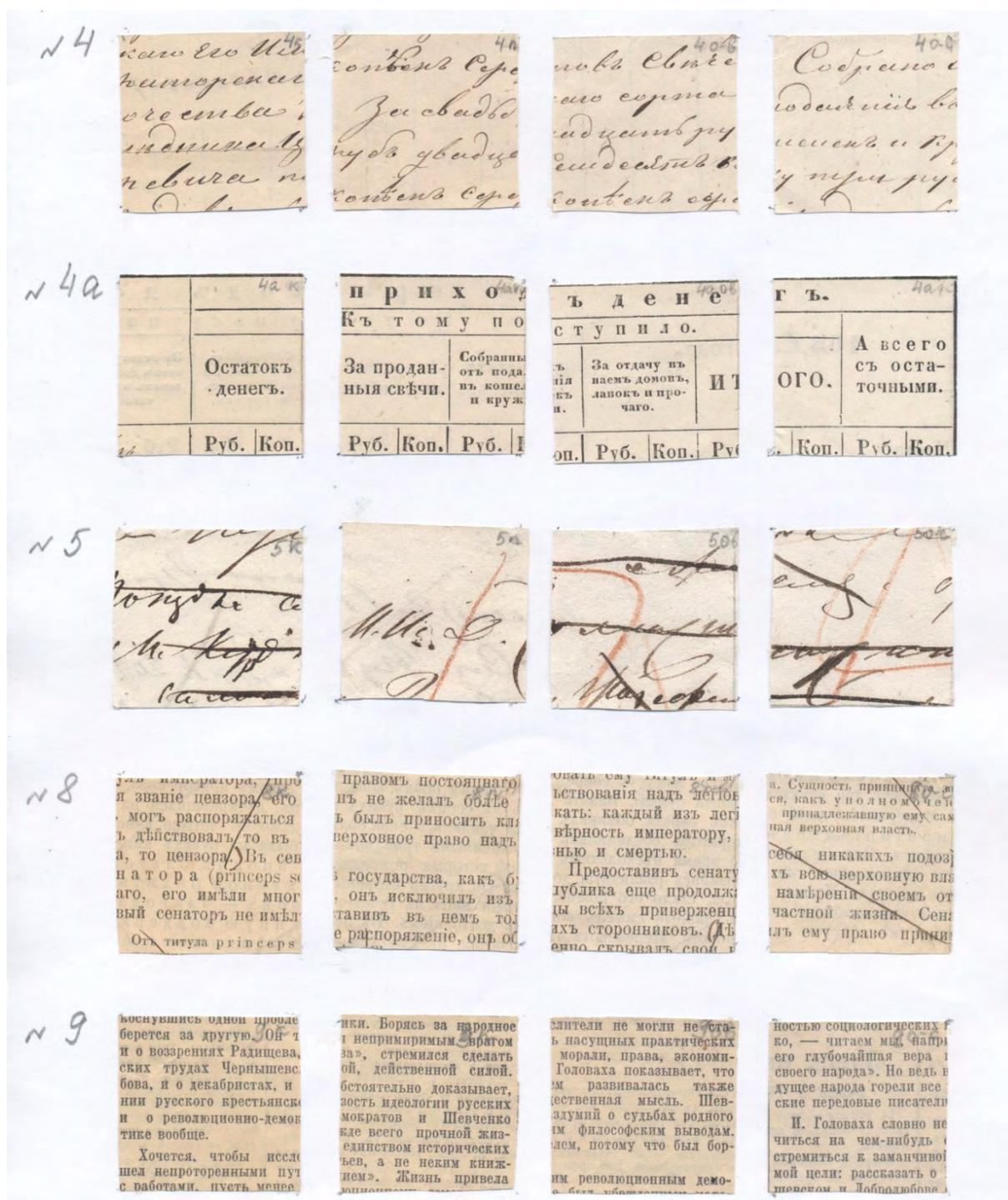
**Fig. 4:** Samples with text: column 1 – control, 2 – washed, 3 – bleached in filtered water, 4 – bleached in water-ethanol mixture
