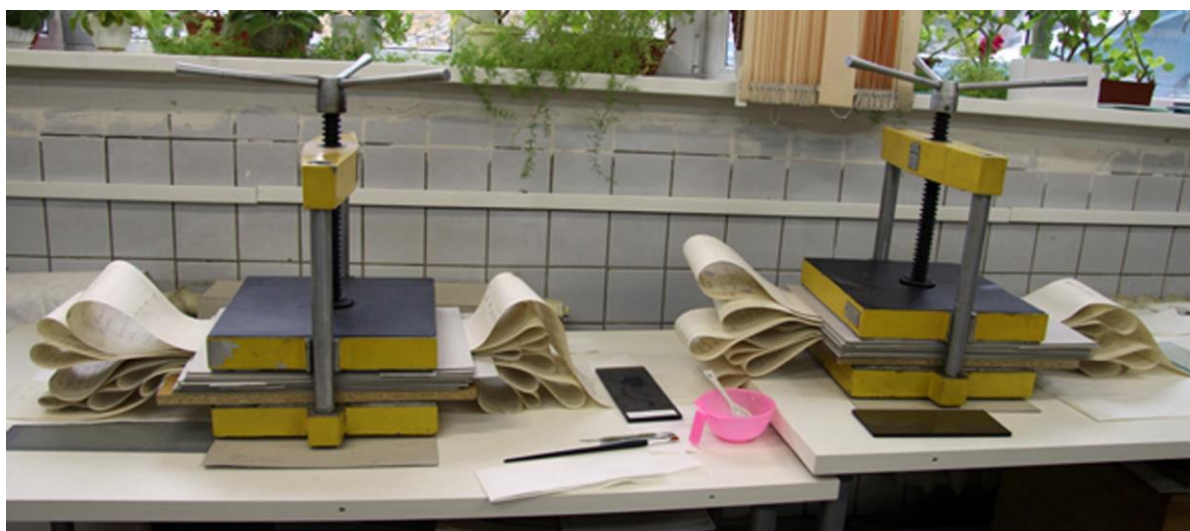
Fig. 11: Several glued sheets were stacked together, sandwiched by cardboard and felt layers and kept under pressure until dry.
